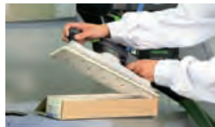
Slippappersbyte – enkelt tack vare StickFix.
